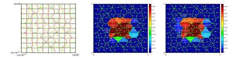
FIGURE 22. Left Superposition of OLD (cartesian) and NEW mesh (truly conic), initial data is given in Figure 11. Comparison of two schemes: center single zone flux scheme (23) and self-intersection scheme (26) on right, slightly difference here, maximum principle obtained in each case (here little white squares represent control points of conic edges).
