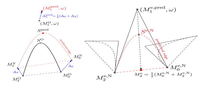
FIGURE 24. Rezoning of control points. Predictor displacement  $\Delta_1^{\text{pred}} = \frac{1}{2}(\Delta_0 + \Delta_2)$ , and Corrector: Predicted control point projected on relaxed position of middle logical edge and Shoulder point of predicted Edge.
