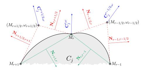
FIGURE 8. Decomposition of vector  $\mathbf{C}_{j}^{\mathrm{dof},\omega}$  at degree of freedom (for short: dof = nodes and control points) for conic cells,  $\mathbf{C}_{j}^{\mathrm{dof},\omega} = \nabla_{M_{\mathrm{dof}}} |C_j|$ .
