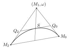
FIGURE 5. Shoulder point of rational quadratic Bezier curve (7).
