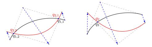
FIGURE 17. Self-intersection for arbitrary conic: at most two intersection points to compute, depending on nodal/control point displacement and weight  $\omega(t)$  evolution.
