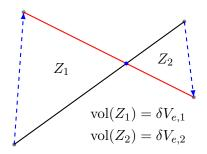
FIGURE 16. Self-intersection for straight polygonal: always at most one intersection point and two sub-areas to compute.
