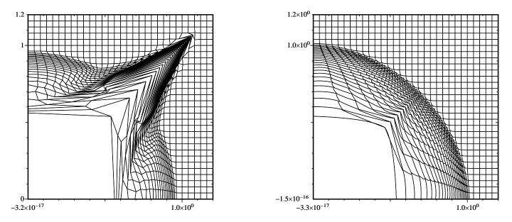
FIGURE 28. Initial logical mesh made by  $30 \times 30$  cells. Meshes at final time for first-order original polygonal GLACE scheme (left) and new conical  $\omega$ -GLACE scheme (right).
