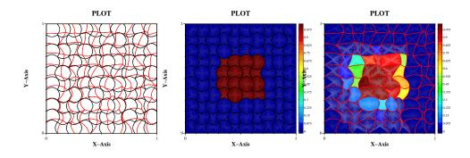
FIGURE 13. Large displacement field test for first-order fluxing scheme (23). Left: superposition of meshes before/after (black/red) rezoning. Center: Initial mesh and data. Right: Final mesh (with modification of weights  $\omega$ ) and solution. Here sub-cycling is needed (4 cycles) because of large displacement, nevertheless maximum principle is still maintained.
