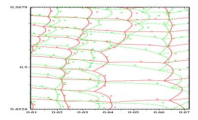
FIGURE 26. Smoothing of conic unstructured cells (arbitrary number of edges) using [ESCO] for node displacement (on polygonal mesh without control points) and a posteriori control point displacement using check of cell validity, Old cells: dashed line (green) with control point represented by (green) dashed circle and New cells: solid line (red) with control point represented by (red) solid square.
