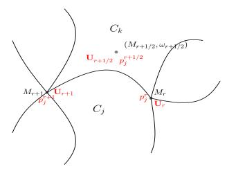
FIGURE 27. Degree of freedom for Lagrangian  $\omega$ -GLACE scheme on conic cell.
