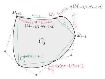
FIGURE 7. Generic cell  $C_j$  and its inclusion in the convex hull of logical polygonal with (in red dashed line) and without (in green polyline) control point (here  $\ell_{a,b}$  is the euclidean distance between point a and b).
