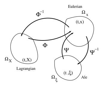
FIGURE 1. Different coordinate system at same time t,  $\mathbf{x} = \Phi(t, \mathbf{X})$  and  $\mathbf{x} = \Psi(t, \xi)$ . The trajectory of a particule in  $\Omega_{\mathbf{x}}$  is defined by  $\frac{d}{dt}\mathbf{x} = V(t, \mathbf{x})$  (with  $\mathbf{x}(0) = \xi$ ).
