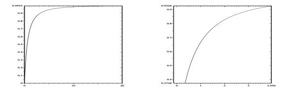
FIGURE 6. Left: graph of the nonlinear function  $f(\omega)$  weighting the area of simplex  $(M_0, M_1, M_2)$  in formula (12)(13), in abscissa weight  $\omega$ . Right: zoom near  $(\omega = 1, f(1) = \frac{2}{3})$ .
