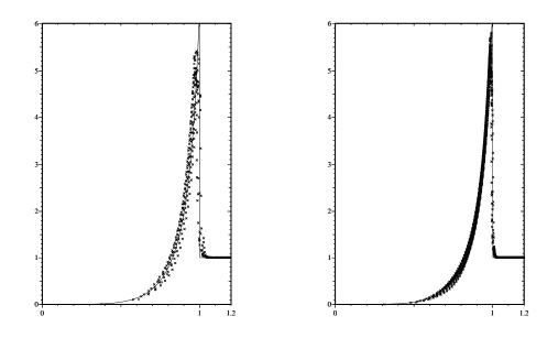
FIGURE 30. Density in all cells as functions of the cell-center at final time for first-order  $\omega$ -GLACE scheme with  $30 \times 30$  logical cells (left) and  $60 \times 60$  cells (right), reference solution in solid line.
