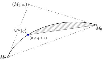
FIGURE 19. Self-intersection computation: Primitive of conic at arbitrary value parameter q gives the area of shaded region.
