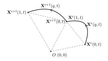
FIGURE 2. Decomposition of boundary integral for area computation.
