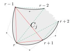
FIGURE 23. Definition of short-medium range same as logical underlying polygonal mesh: Short  $r = \{r + 1, r - 1\}$ , Med  $r = \{r + 2, r - 2\}$ .
