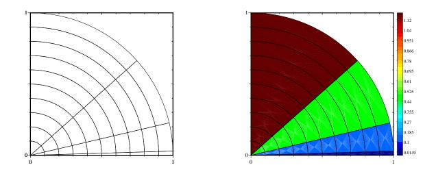
FIGURE 14. Initial circular mesh with non equi-angular sector (left) and initial condition (right).
