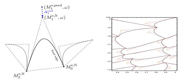
FIGURE 25. Rezoning: Moving node and control point with distance diminution in case of non valid cell (total displacement  $\Delta_1 = \Delta_1^{\text{pred}} + \Delta_1^{\text{cort}}$  (Figure 24 and 25)). Right: dashed line draw the link between control point to both end points and Shoulder point: final conic cells are valid if underlying logical polygon are valid.
