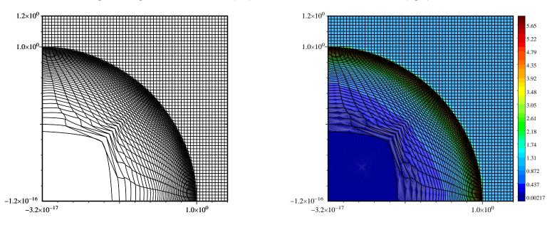
FIGURE 29. Initial Logical mesh made by  $60 \times 60$  cells. At final time, we have depicted the mesh (left) and the numerical solution (right) of the first-order conical  $\omega$ -GLACE scheme.
