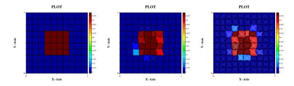
FIGURE 11. Left: Initial data and mesh, Final meshes and solutions of first-order remapping scheme (23) for polygons ( $\omega = 0$ ) on center and ellipse ( $\omega = 0.5$ ) on the right.
