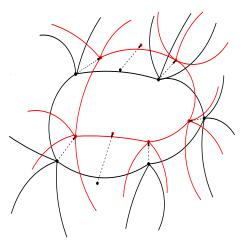
FIGURE 9. Exact geometric problem: computation of conic/conic mesh intersection between old mesh (black) and new mesh (red) after moving nodes, control points and weight re-adjustment.
