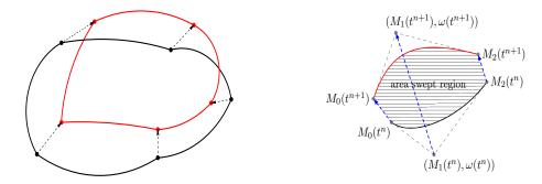
FIGURE 10. Left: Old cell (black) moves to new cell (red); Right: The area swept by edges forms conic cells which can be computed exactly by (14) or (16).
