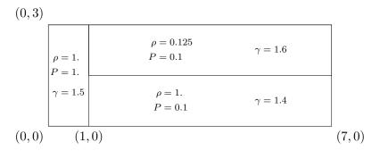
FIGURE 31. Initial regular cartesian grid with  $n_x = 36$ ,  $n_y = 16$ . We take three perfect gases (with different  $\gamma$ ) at rest in three different zones. Control points are initially set in the middle of logical edge.
