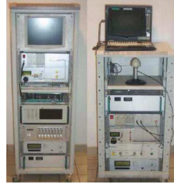
Figure 4. MIMO channel sounder: receiver and transmitter.
