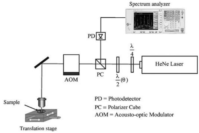
Fig. 12. Schematic diagram of the laser vibrometer bench.
