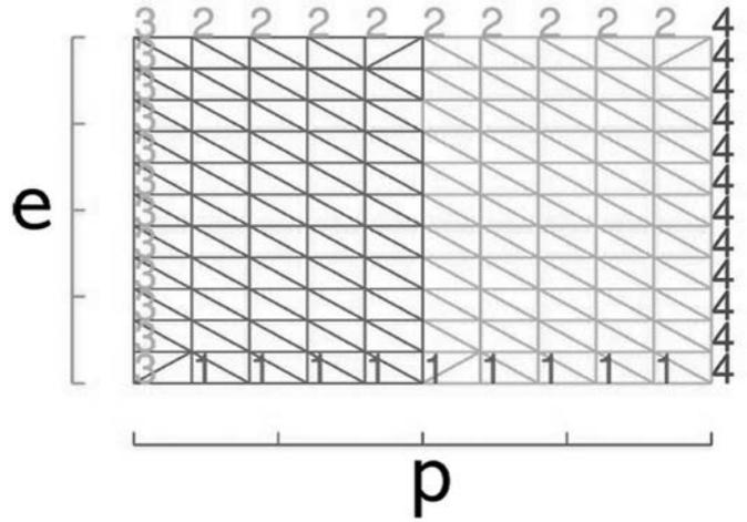
Fig. 2. Two-dimensional mesh of a periodically poled transducer.
