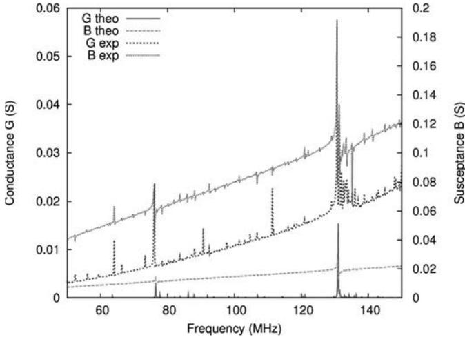
Fig. 5. Comparison between experimental results and theoretical predictions for a 500- $\mu\text{m}$ -thick LiNbO<sub>3</sub> transducer ( $\lambda = 50 \mu\text{m}$ ).
