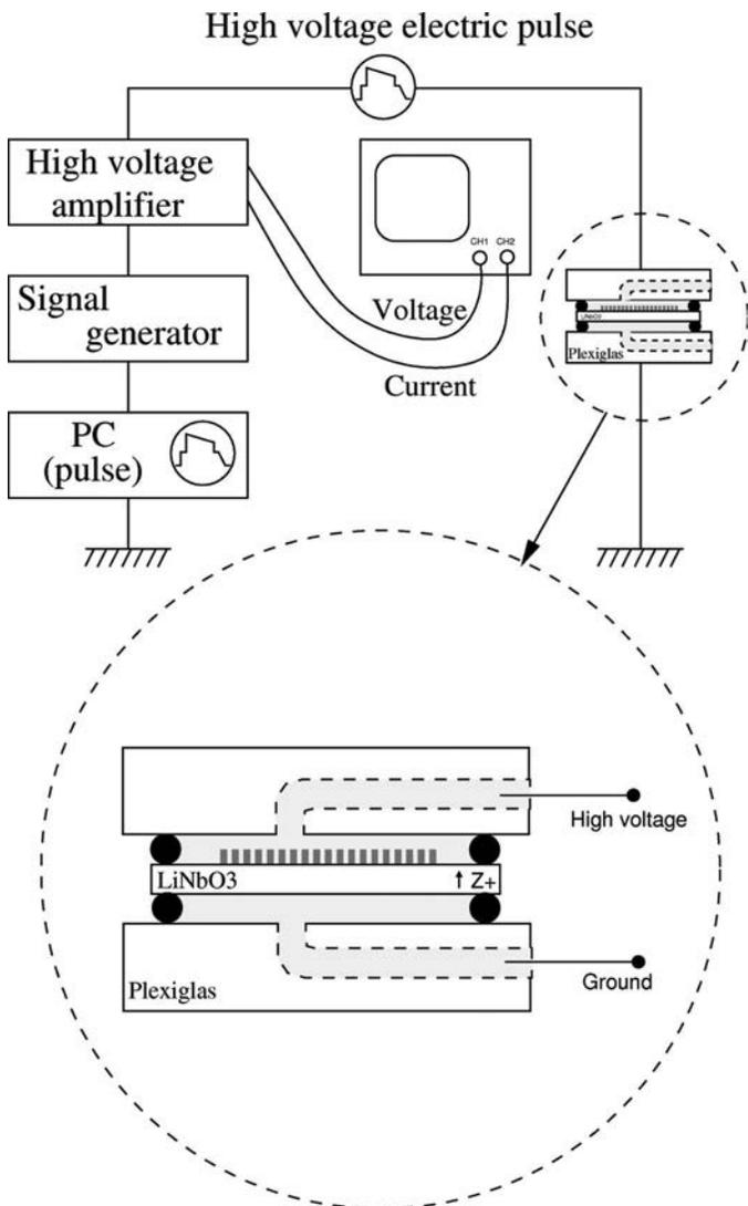
Fig. 4. Schematic diagram of the poling bench.
