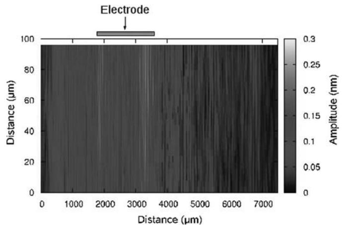
Fig. 13. Acousto-optical scan performed using a laser vibrometer showing the amplitude variation of the vibrations versus the distance.
