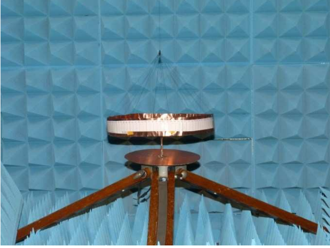
Figure 6: Picture of the experimental set-up showing the suspended detector ring in the anechoic chamber.
