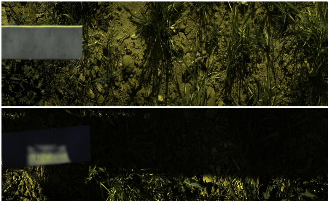
FIGURE 1: Two reflectance images in false RGB colours with different lighting conditions without shadow (up), with shadows (down). On the left : the ceramique plate.
