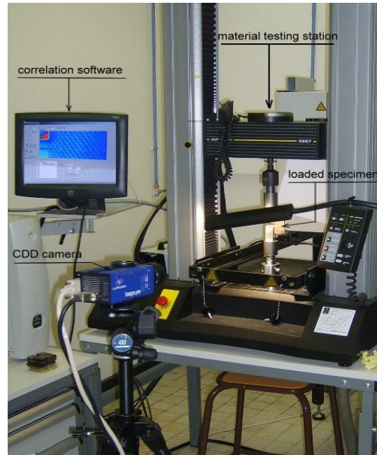
Fig. 5. Experimental set-up and images capture of the CT specimens.
