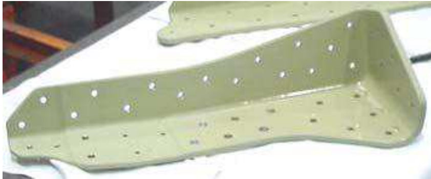
Fig 1: Case corner part used for aeronautical application
