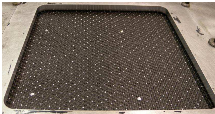
Fig 4: Carbon reinforcement with markers at the initial state
