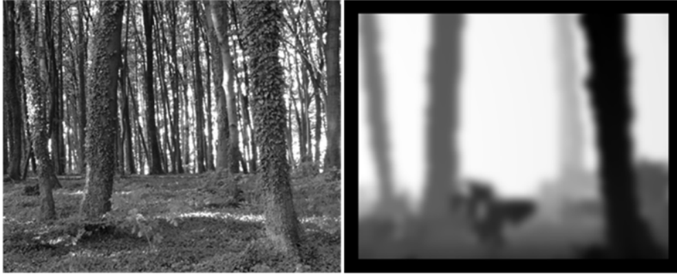
Figure 13: Original picture (a) and its disparity map (black areas stand for the closest areas whereas the bright areas indicate the farthest ones).
