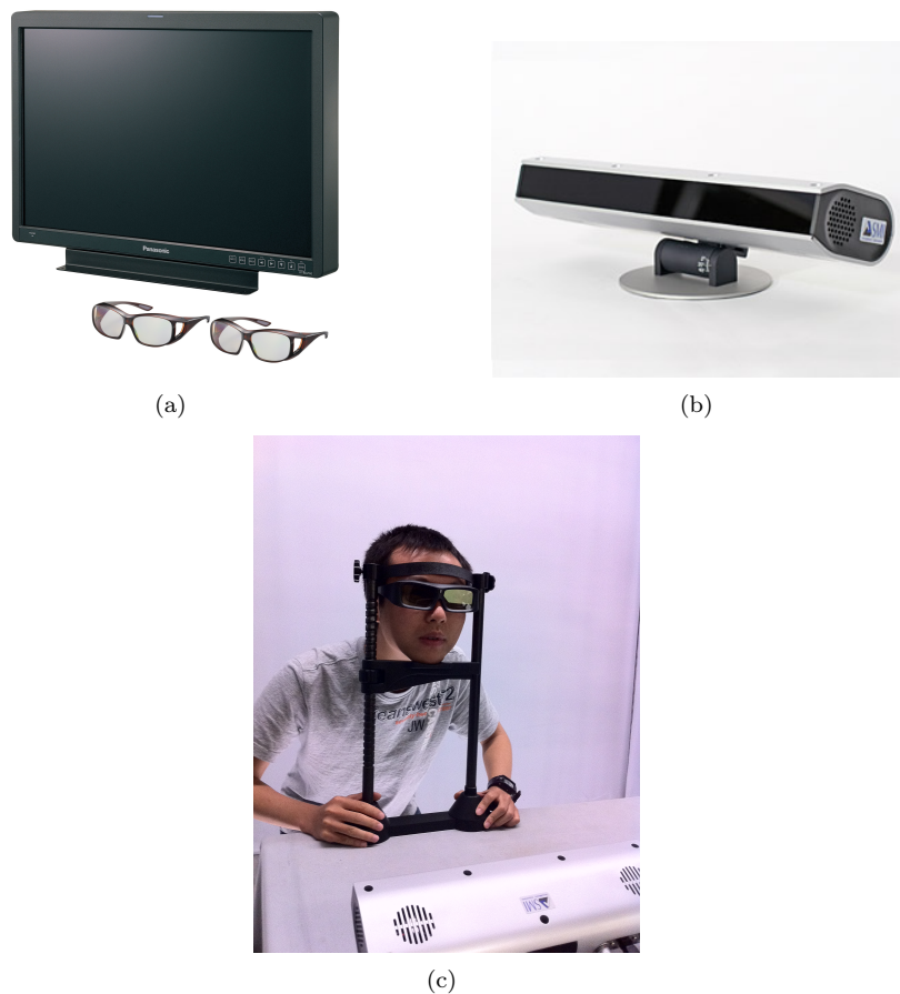
Figure 7: (a)The 26-inch Panasonic BT-3DL2550 LCD screen used in the experiment. (b)SMI
