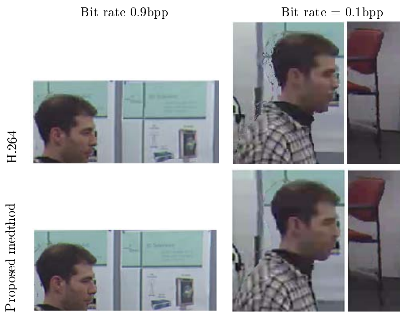
Figure 35: Snapshots of synthesized views from data encoded with H.264 and from data encoded with the proposed method.
