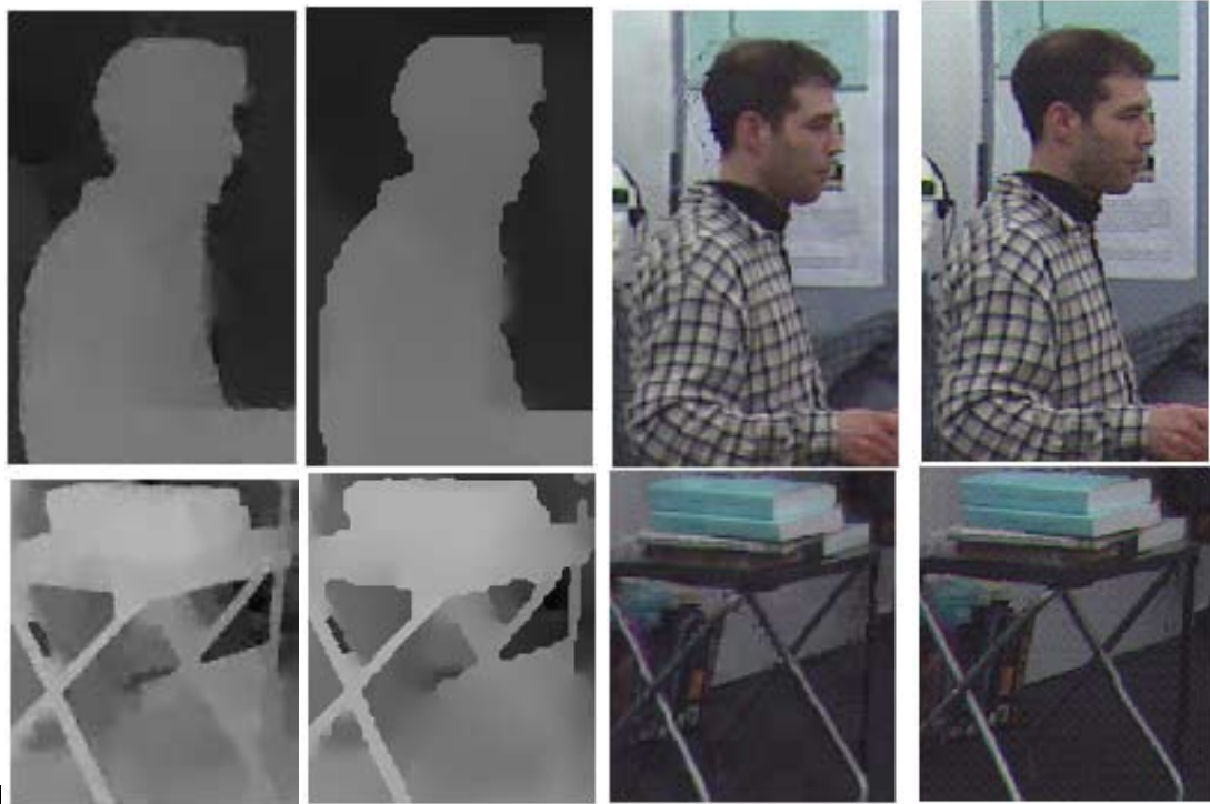
]Decoded depth when applying quantization suggested in Pasteau et al. Decoded depth when applying our proposed strategy. Frame synthesized from decoded depth when applying quantization suggested in Pasteau et al. Frame synthesized from decoded depth when applying our proposed strategy.
