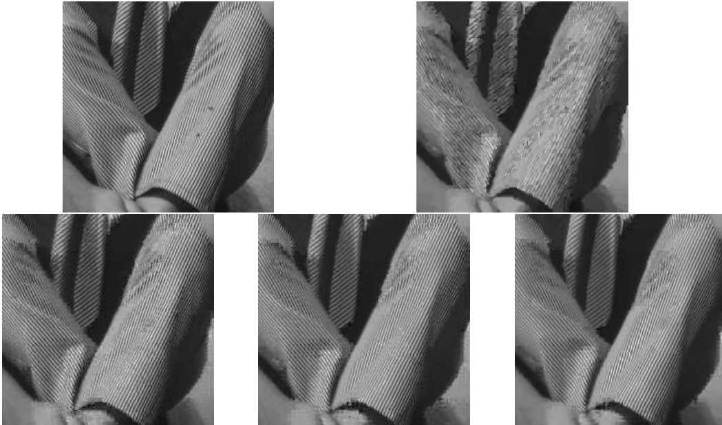
Figure 2.7: Prediction results for a textural region of Barbara image at low bit-rates ( q_f = 10 ). (a) Original image, (b) H.264 intra modes, (c) SP, (d) LLE, and (e) NMF based prediction methods with MSE criterion and sparsity constraints ( k \in [1, 8] ).
