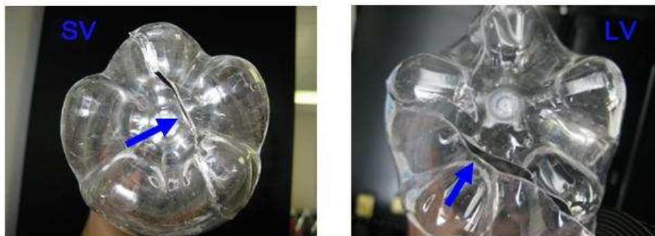
Figure 2: Probability density function for the “time before cracking” variable. The LV base resists much better than the SV one. In both case, the crack initiate in the circumferential direction, between a foot and the injection point.
