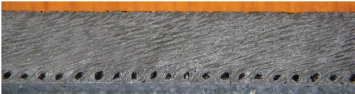
Figure 10: Cross section of a tube manufactured by radial injection moulding (4 preferential channel mould)
