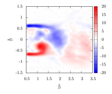
Figure 10: Snapshot of the vorticity field reconstructed from the reduced order model estimated through the strong constraint assimilation of the LES data (a) and the PIV data (b).
