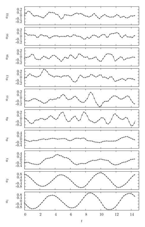
Figure 12: Reconstructed temporal modes trajectories for the PIV sequence showing 3 vortex shedding (256 snapshots): dashed line, the data (every 2 snapshots instants); solid line, results of the weak constraint assimilation.
