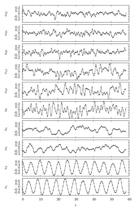
Figure 13: Reconstructed temporal modes trajectoß fs for the PIV sequence showing 12 vortex shedding (512 snapshots): dashed line, the data (every 4 snapshots instants); solid line, results of the weak constraint assimilation.
