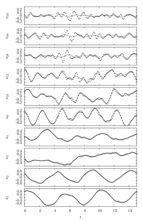
Figure 7: Reconstructed temporal modes trajectordes for the LES sequence showing 3 vortex shedding (256 snapshots): dashed line, the data (every 2 snapshots instants); solid line, results of the strong constraint assimilation.
