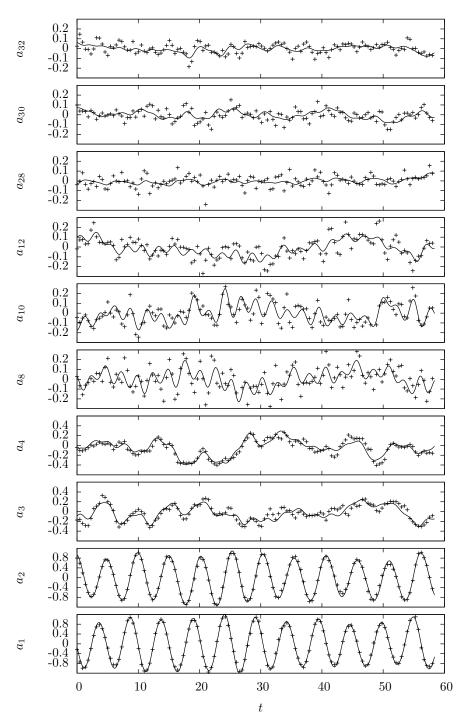
Figure 9: Reconstructed temporal modes trajector **26** for the PIV sequence showing 12 vortex shedding (512 snapshots): dashed line, the data (every 4 snapshots instants); solid line, results of the strong constraint assimilation.
