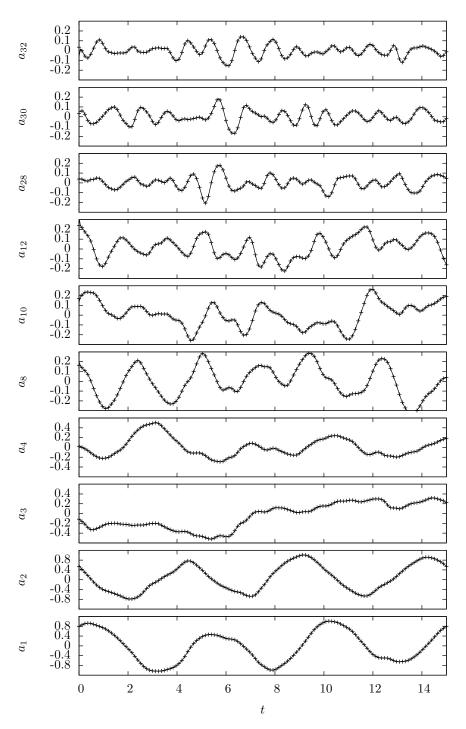
Figure 11: Reconstructed temporal modes trajectors for the LES sequence showing 3 vortex shedding (128 snapshots): dashed line, the data (every 2 snapshots instants); solid line, results of the weak constraint assimilation.
