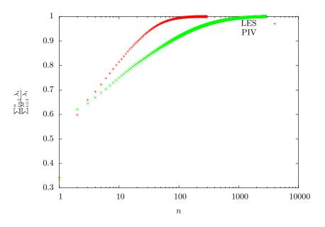
Figure 6: Cumulative turbulent kinetic energy distribution with respect to the number of modes for the 300-snapshots LES sequence (red curve) and the  $3\,072$ -snapshots PIV sequence (green curve).
