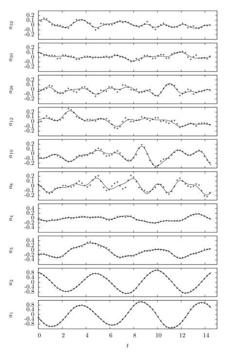
Figure 8: Reconstructed temporal modes trajecto25 for the PIV sequence showing 3 vortex shedding (128 snapshots): dashed line, the data (every 2 snapshots instants); solid line, results of the strong constraint assimilation.
