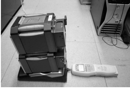
(a) Experimental setup for measuring the friction coefficient between the foot and the floor.
