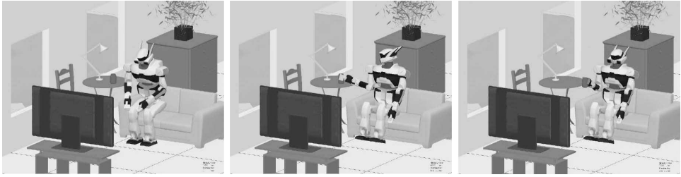
Fig. 6. HRP-2 sitting in a sofa and taking a can. This simulation shows a realistic scenario in a complex environment with robust multi-contact resolution.
