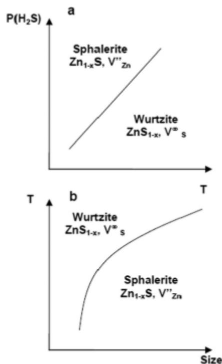
**Figure 10 : Schematic representations of ZnS sphalerite–wurtzite phase transition, (a)<sup>36–38</sup> as a function of temperature and P(H<sub>2</sub>S), (b)<sup>40</sup> as a function of temperature and ZnS crystal size.**
