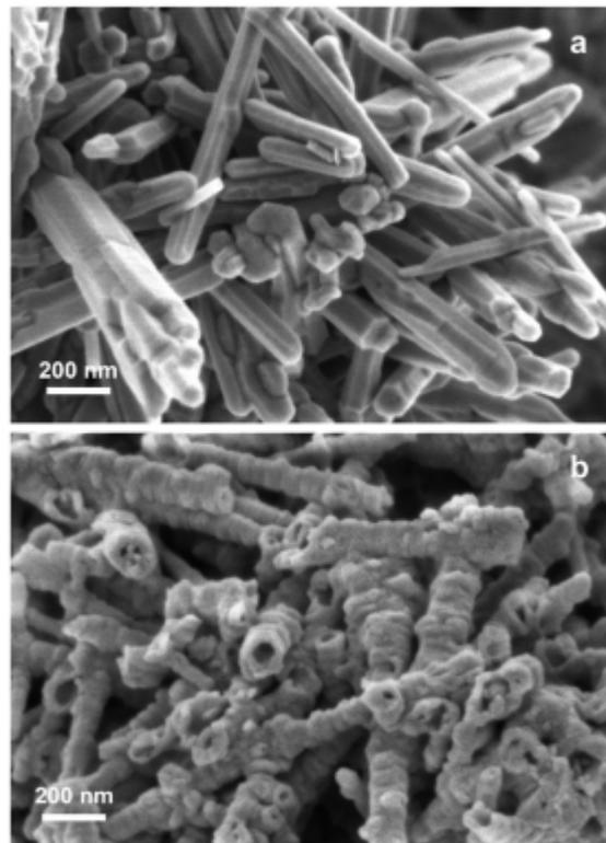
Figure 3: SEM micrographs of ZnO particles: (a) before sulfidation and (b) after sulfidation at 295°C and P(H<sub>2</sub>S)=10 kPa ( $\alpha=0.9$ )
