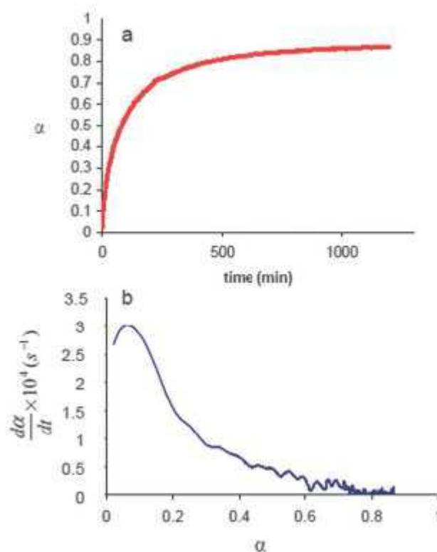
**Figure 1 : (a) variation of the fractionnal conversion versus time of ZnO sulfidation at 310°C, P(H<sub>2</sub>S)=5kPa and P(H<sub>2</sub>O)=2,5kPa. (b) variation of the reaction rate  $d\alpha/dt$  as a function of fractionnal conversion  $\alpha$ .**
