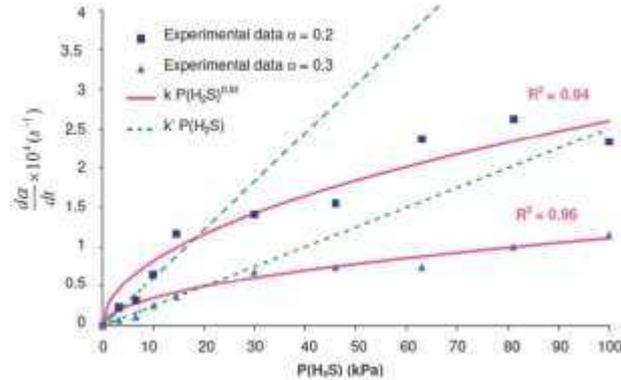
**Figure 14 : Variation of the kinetic rate versus  $P(\text{H}_2\text{S})$  of ZnO sulfidation for the same fractional conversion ( $\alpha=0.2$  and  $\alpha=0.3$ ) at 260°C,  $P(\text{H}_2\text{S})$  variable up to 100 kPa,  $P(\text{H}_2\text{O})=1.8$  kPa.**
