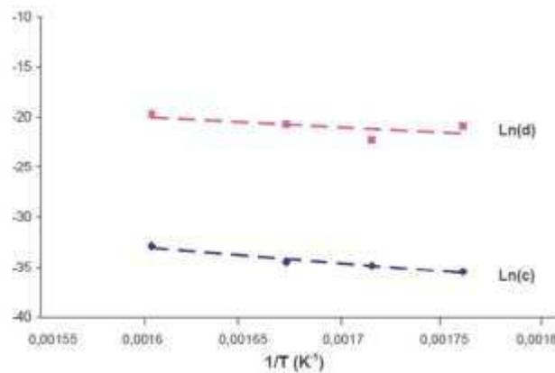
**Figure 18 : Representation of Ln(c) and Ln(d) functions of 1/T for ZnO sulfidation reaction at various temperatures 295–310–325–350°C, P(H<sub>2</sub>S)=5 kPa, P(H<sub>2</sub>O)=2.5 kPa, where c and d are the values expressed in eqn (14).**
