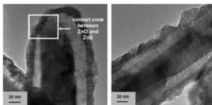
Figure 4: TEM micrographs of partially sulfided ZnO particles ( $\alpha=0.3$ ) at 230°C, P(H<sub>2</sub>S)=5 kPa and P(H<sub>2</sub>O)=2.5 kPa
