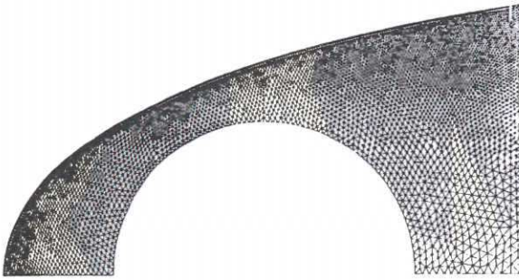
Fig. 4. - Mesh of part of the generatrix plane: elastic shell and part of the internal fluid domain.
