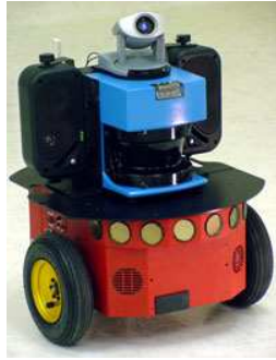
Fig. 5 Robot Test-bed; an ActiveMedia Pioneer 2-DX mobile robot equipped with a SICK laser range scanner, a camera, and speakers.
