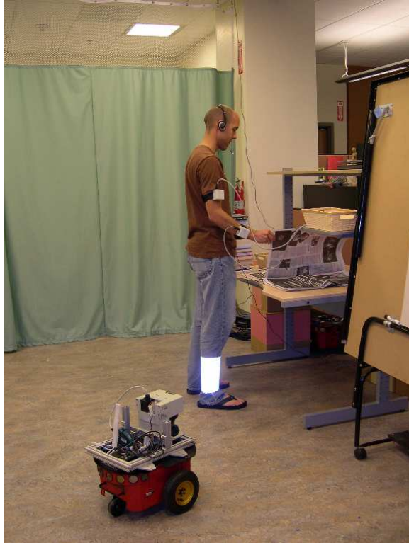
Fig. 6 The first experimental setup: the participant is performing Task 4 (turning pages of a newspaper) with the robot at a social distance. The laser fiducial is on the participant’s right leg, the motion sensor on the right arm, and a microphone is worn on standard headphones.
