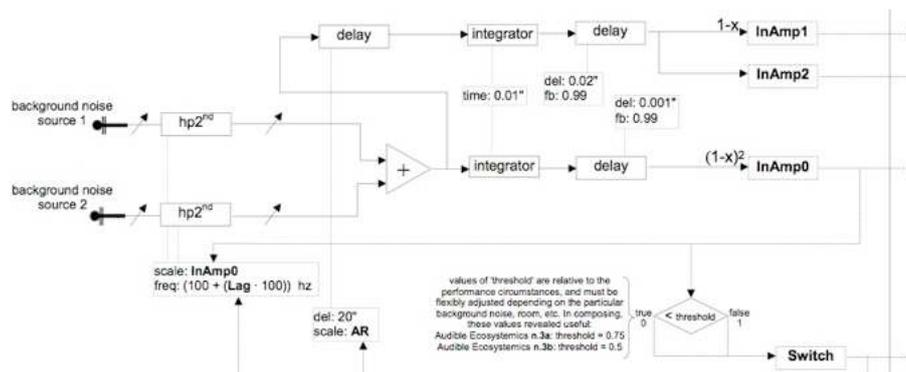
**Figure 2.** Part of the DSP schema for *Audible ecosystems 3a/3b* [Di Scipio, 2004-2005: 6]. On this figure, we can see a loop: [Hp2nd] → [integrator] → [delay] → [InAmp0] → [scale: InAmp0 / freq: (100+(lag·100))hz] → [Hp2nd].
