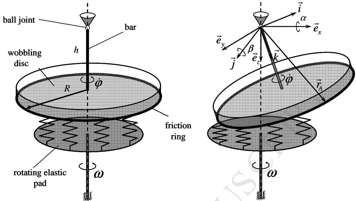
**Fig. 1.** Rotating friction disc on the elastic pad and the corresponding coordinate systems
