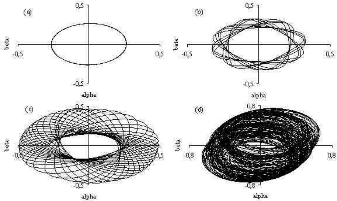
**Fig. 10.** Limit cycles obtained by numeric simulations: (a) – stable limit cycle with regular precession for the slip  $\omega - \dot{\varphi} = 70 \text{ rad/s}$ , (b) – more complex limit cycle for  $\omega - \dot{\varphi} = 75 \text{ rad/s}$ , (c) – the next complexity level for  $\omega - \dot{\varphi} = 105 \text{ rad/s}$ , (d) – seemingly chaotic behavior for  $\omega - \dot{\varphi} = 220 \text{ rad/s}$
