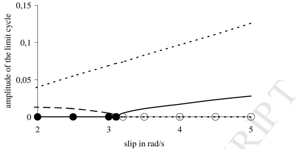
**Fig. 7.** Transcritical bifurcation in the disc's dynamics; stable equilibrium – solid line with solid dots, unstable equilibrium – dotted line with circles, stable periodic solution – solid line, unstable branch of the same periodic solution – dashed line, unstable periodic solution – dotted black line.
