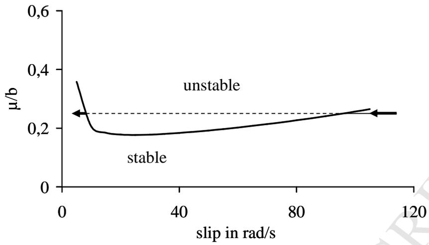
**Fig. 5.** Alternation of stable and unstable domains while synchronizing the disc
