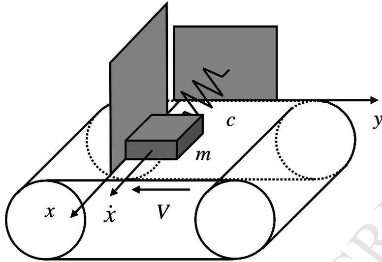
**Fig. 2.** A mass on the moving belt
