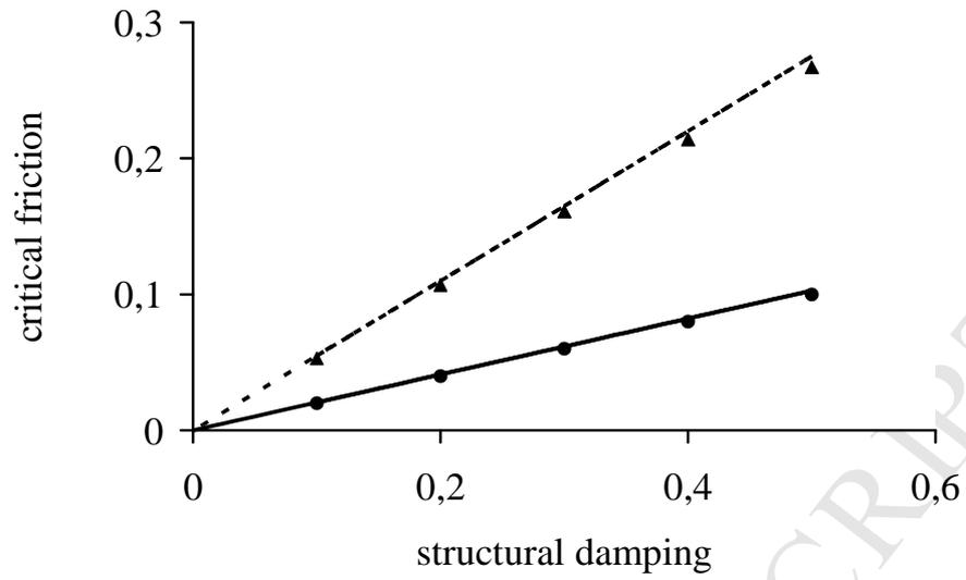
**Fig. 4.** Critical friction as a function of the structural damping for positive slip (solid line) and negative slip (dashed line); dots and triangles correspond to the numeric simulations of the nonlinear equations
