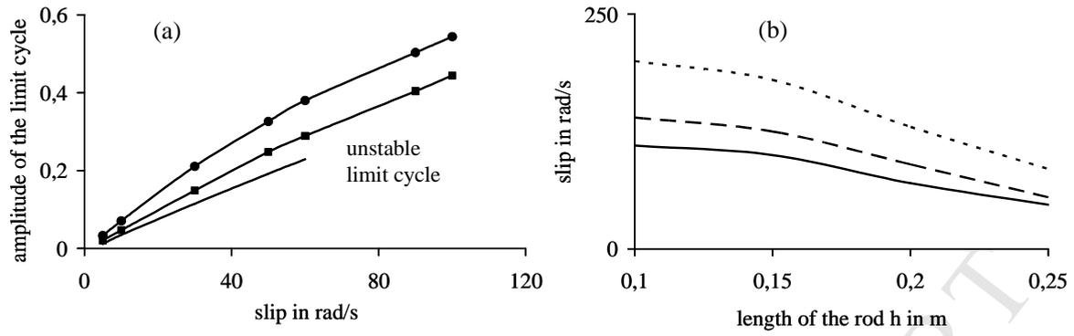
**Fig. 9.** Limit cycle and its stability domain; (a):  $h=0,1$  for the line with circles,  $h=0,15$  for the solid line with crosses,  $h=0,2$  for the solid line; (b):  $\omega = 100 \text{ rad} / \text{s}$  for the solid line,  $\omega = 200 \text{ rad} / \text{s}$  for the dashed line,  $\omega = 300 \text{ rad} / \text{s}$  for the dotted line
