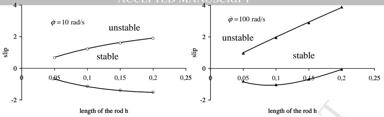
**Fig. 3.** Stability domain of the undamped system; solid line – stability boundary according to (21), circles/dots – stability boundary according to numeric simulations of the complete equations (3) – (12)
