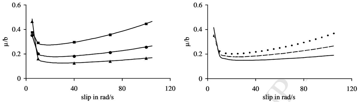
**Fig. 6.** Friction/damping threshold as a function of the design parameters; (a)  $h=0,1$  for quads,  $h=0,15$  for dots,  $h=0,2$  for triangles; (b) dotted line for  $c=15.000$  N/m, dashed line for  $c=30.000$  N/m, solid line for  $c=60.000$  N/m
