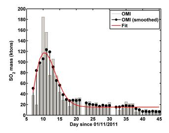
**Fig. 7.** Time series of SO<sub>2</sub> total mass measured with OMI for the 2011 eruption of Nyamulagira. Shown are the daily values (grey), 5-day moving averages (black) and a skewed shape function fitted to the smoothed curve (red).
