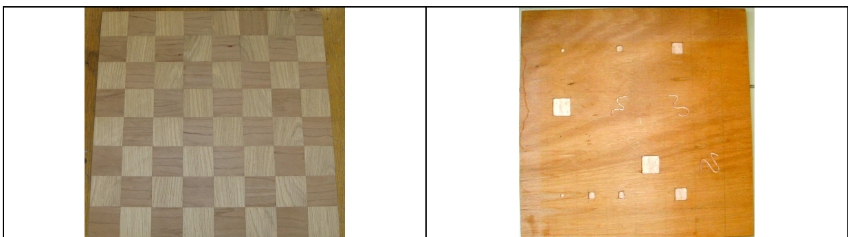
Figure 13: The analyzed academic chess-board (on the left) and the location of the defects (on the right)
