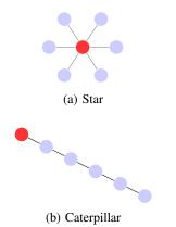
Fig. 8: Extreme cases of average branching factor and the corresponding tree topology.
