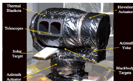
Figure 1 – The MRO/MCS instrument during thermal vacuum testing at JPL
