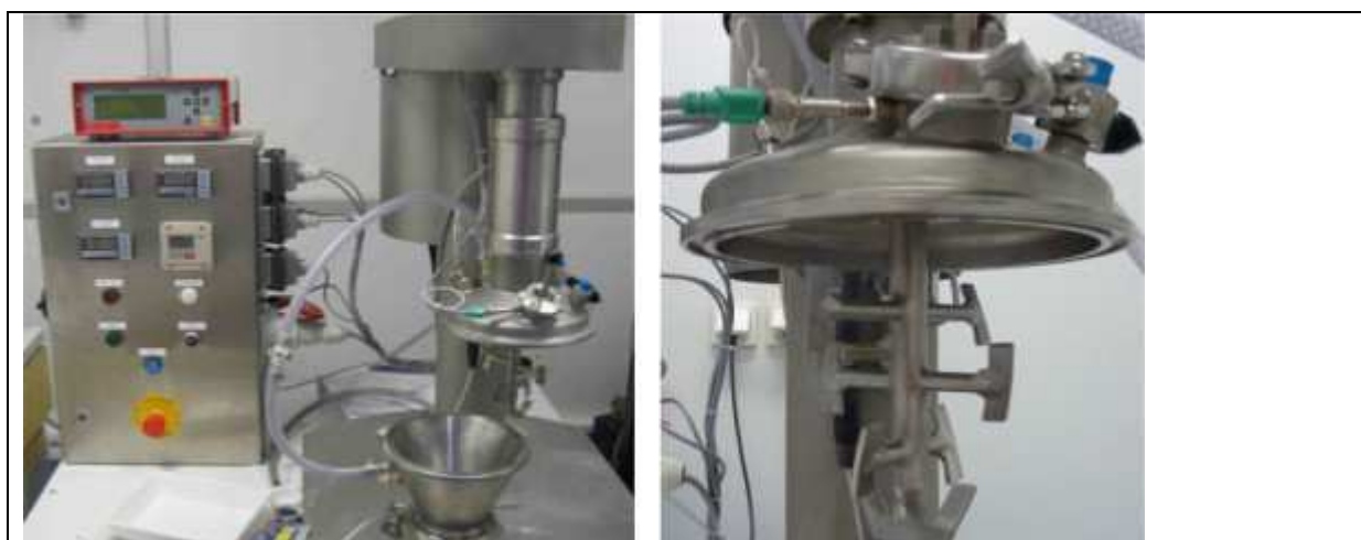
Figure 3: Cyclomix high shear mixer lab-scale device.
