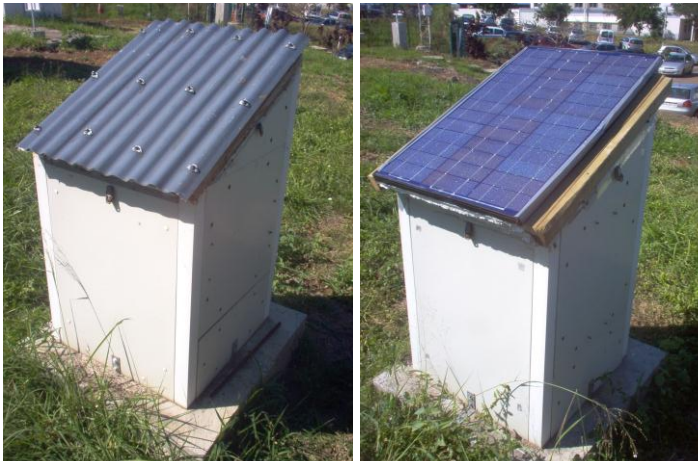
Fig 9. Photography of Isotest cell without and with PV panel
