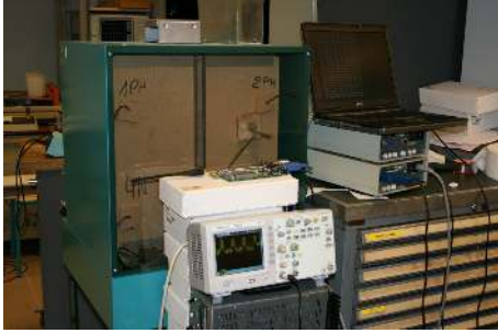
Figure 7. High temperature bench : ceramic oven with non-metallic back for RF wireless measurement associated with oscilloscope for debugging signal issue from reader unit, another temperature probe is used to measure temperature as close as possible of the device.
