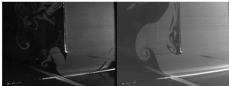
(a) \Delta T_{1/2}=27,6\text{K} ( Fr=1,95 ) (b) \Delta T_{1/2}=11,4\text{K} ( Fr=4,7 )
