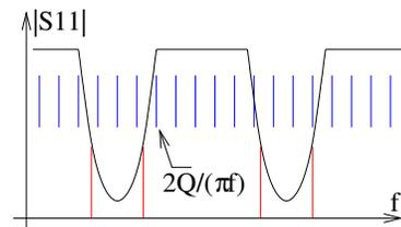
Figure 5. For a dual-mode resonator, required for a differential measurement, a minimum of 4 measurements each lasting  $2Q/(\pi f)$  seconds, with  $f$  the resonance frequency of one mode and  $Q$  its quality factor, is needed (red). A more classical approach of a frequency sweep network analyzer requires up to 128 measurements in the 434-MHz European ISM band (blue).
