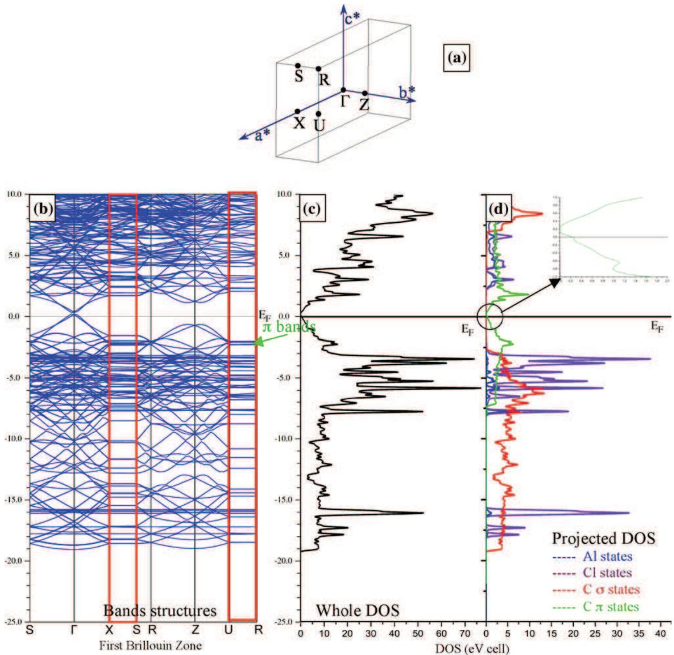
**Fig. 5**  $\text{AlCl}_3\text{-GIC}$  bands structure results. **a** First Brillouin Zone. **b** Bands structure diagram. **c, d** Whole and projected DOS. The absence of dispersion (flat bands) along the directions parallel to  $\vec{c}$
