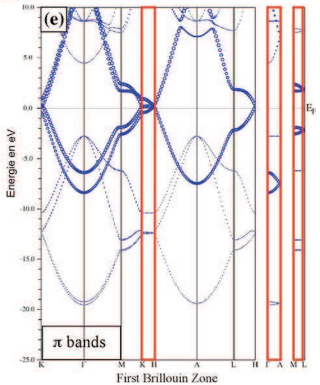
◀ **Fig. 4** **a** Bands structure diagrams. **b** whole and projected DOS for graphite. **c** First Brillouin Zone. **d, e** Fat bands diagrams emphasizing in thick lines the  $\sigma$  and  $\pi$  bands contributions. The superimposed *red* rectangles point out the directions parallel to  $\vec{c}$  axis along which the bands dispersions are associated to orbitals overlaps through the van der Waals gap (Color figure online)
