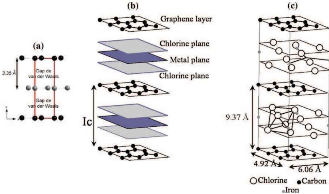
**Fig. 2** Schematic representation of the structure of graphite and  $MCl_x$ -GICs. In the case of graphite (a) the interlayer spacing is 3.35 Å. In the case of GICs (b) the van der Waals gap is occupied by
