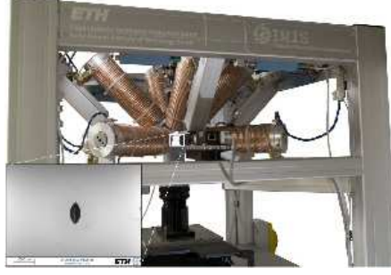
Fig. 7 The OctoMag electromagnetic system. 8 soft-magnetic-core electromagnets surround the arena containing the micro-robot. A camera is fitted down the central axis to image the micro-robot [21].
