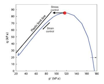
Figure 1. Typical undrained biaxial behavior of a loose sand. At the *q*-peak, following the axial control parameters, the specimen can liquefy (strain control) or can give rise to a sudden failure (stress control). From Darve *et al.* [15].
