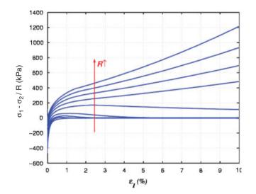
Figure 3. Proportional strain triaxial loading paths. From Darve et al. [15].
