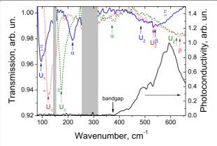
**Figure 6 Typical CR spectra and photoconductivity spectrum for sample 3.** The numbers against the CR lines are the magnetic field values in Tesla. Arrows indicate the observed cyclotron peaks. Gray stripes are Reststrahlen bands. The 'bandgap' mark indicates the value of the bandgap for 4.8-nm HgTe QW.
