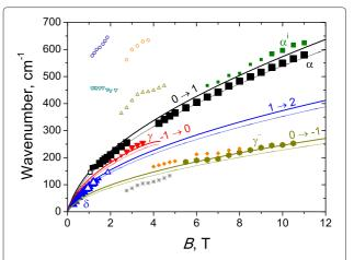
**Figure 5** Energies of cyclotron transitions versus the magnetic field for sample 2. Solid lines correspond to the calculated transitions with adjusted parameters; thin dotted lines, with traditional parameters. Symbols are experimental data. The size of symbols indicates the intensity of CR lines: the smallest symbols correspond to weak lines.
