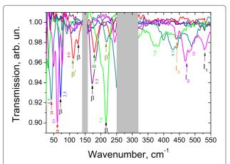
**Figure 2 Typical CR spectra for sample 1.** The numbers against the CR lines are the magnetic field values in Tesla. Gray stripes are Reststrahlen bands.
