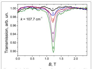
**Figure 4 Typical CR spectra for sample 2 measured using 3.2-THz QCL.** In the absence of visible light illumination (1) and at various levels of illumination (2 to 5). The carrier density in units of  $10^{10}$  cm<sup>-2</sup> is 3.5 (1), 5.4 (2), 7.2 (3), 9.3 (4), and 10.3 (5).
