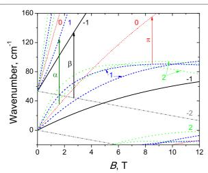
**Figure 1** Calculated Landau levels for sample 1 using the adjusted parameters. Integers denote the number *n* of the Landau levels. Vertical arrows indicate the experimentally observed transitions.
