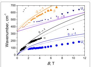
**Figure 7** Energies of cyclotron transitions versus the magnetic field for sample 3. Solid lines correspond to the calculated transitions with adjusted parameters; thin dotted lines, with traditional parameters. Symbols are experimental data. The size of symbols indicates the intensity of CR lines: the smallest symbols correspond to weak lines.
