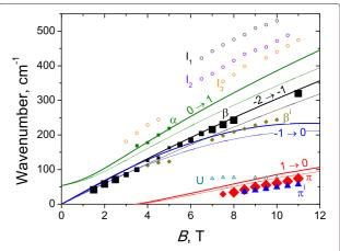
**Figure 3** Energies of cyclotron transitions versus the magnetic field for sample 1. Solid lines correspond to the calculated transitions with adjusted parameters; thin dotted lines, with traditional parameters. Symbols are experimental data. The size of symbols indicates the intensity of CR lines: the smallest symbols correspond to weak lines.
