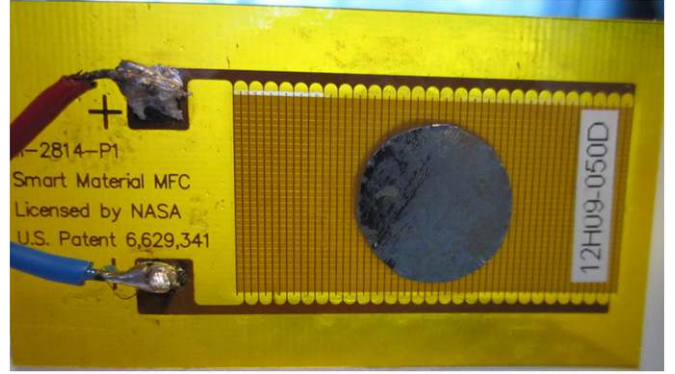
Figure 5. 10 mm FeSiB metglass disks glued on both sides of a single MFC.
