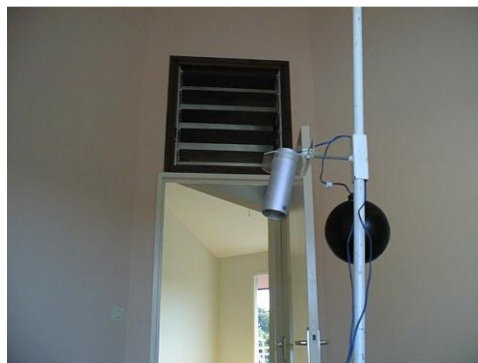
Fig. 9 : Measurements of ambient air and resultant temperature inside dwelling
