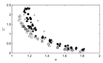
Fig. 6. Undimensional sheet cavity length  $L^* = L/H_{throat}$  according to the cavitation number  $\sigma$ :  $\times$ : plate 0,  $\bigstar$ : plate 1,  $\triangle$ : plate 2,  $\blacktriangle$ : plate 3, +: plate 4,  $\bigstar$ : plate 5, +: plate 6,  $\diamondsuit$ : plate 7,  $\square$ : plate 8.
