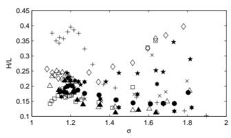
Fig. 8. Aspect ratio H/L according to the cavitation number  $\sigma$ :  $\times$ : plate 0,  $\bigstar$ : plate 1,  $\triangle$ : plate 2,  $\star$ : plate 3, +: plate 4,  $\bigstar$ : plate 5, +: plate 6, star: plate 7,  $\square$ : plate 8.
