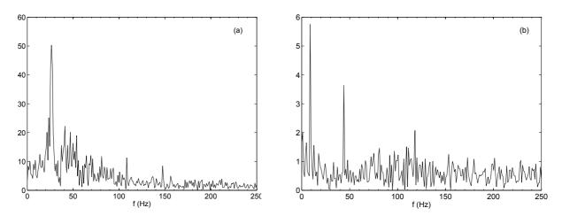
Fig. 11. Frequency spectrum of the variation of the gray level in the closure of the sheet cavity, on the plate 0: (a) for  $\sigma = 1.17$ , (b) for  $\sigma = 1.44$
