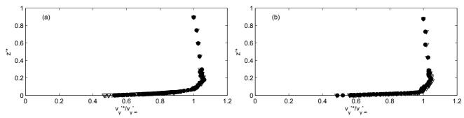
Fig. 16. Longitudinal non-dimensional velocity profile  $v_y'^*/v_{y_\infty}'$  of the non-cavitating flow, at  $y^*=0.5$ , for (a) the grooved sheet 6 and (b) the grooved sheet 2.  $\bullet$ :  $x^*=0$ ,  $\triangle$ :  $x^*=\frac{\lambda}{2}$
