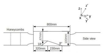
Fig. 1. Test section of the experimental device using a Venturi profile (the origin of the cartesian coordinate system is located at the throat, in the middle of the test section wide,  $\alpha = 8^{\circ}$  is the angle for the LDV measurements system xy'z' and  $H_{throat} = 67 \,\mathrm{mm}$  is the reference length).
