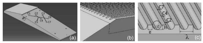
Fig. 3. Venturi components: (a) Venturi basis with C1 to C7 pressure sensors on the basis surface, (b) junction between the Venturi basis and a plate and (c) zoom of a grooved plate with the definition of the grooves geometric parameters (d and h are respectively the grooves diameter and depth, e is the width of the ridge and  $\lambda$  is the grooves wavelength).
