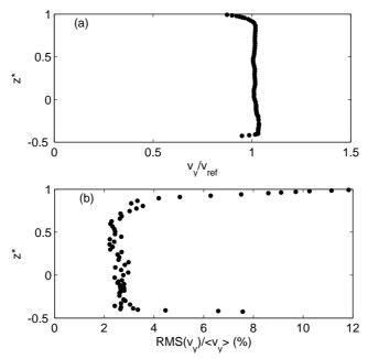
Fig. 2. Characterisation of the flow in the test section inlet: (a) undimensional longitudinal velocity profile  $v_y^* = v_y/v_{ref}$  (the line represents the mean value of the velocity  $v_{ref} = 5.56\,\mathrm{m.s^{-1}}$ ) and (b) the profile of the turbulence intensity  $\frac{RMS(v_y)}{< v_y>}$ , where  $< v_y>$  is the time-averaged velocity,  $y^* \simeq -4.5$  and  $x^* = 0$  (Results come from LDV measurements, presented in the section 4.1).
