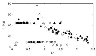
Fig. 10. Frequency of the sheet cavity length oscillation  $f_L$  according to the undimensional sheet cavity mean length  $L^*$ :  $\times$ : plate 0,  $\bigstar$ : plate 1,  $\triangle$ : plate 2,  $\star$ : plate 3, +: plate 4,  $\star$ : plate 5, +: plate 6,  $\diamondsuit$ : plate 7,  $\square$ : plate 8.
