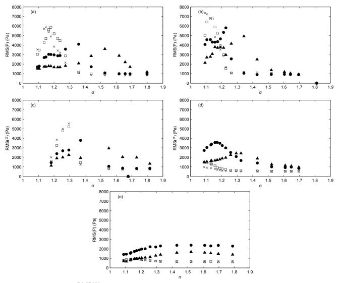
Fig. 9. Pressure fluctuations RMS(P) on the Venturi bottom wall according to the cavitation number  $\sigma$ , at different distances from the ventrui throat:(a) for plate 0,(b) for plate 2, (c) for plate 3, (a) for plate 4, (a
