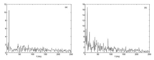
Fig. 12. Frequency spectrum of the variation of the gray level in the closure of the sheet cavity, for  $\sigma = 1.17$  for: (a) the plate 8
