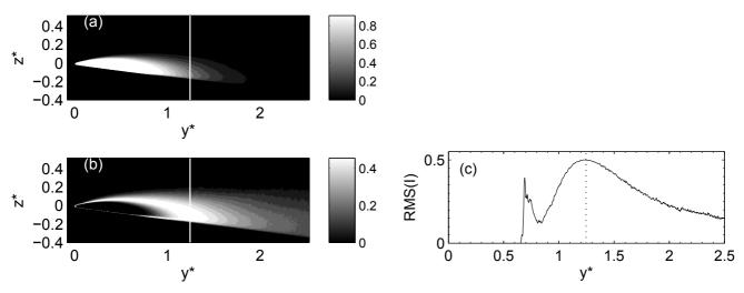
Fig. 5. Sheet cavity on the smooth plate 0 for  $\sigma=1.18$ : (a) normalized average image, (b) root mean square of normalized images (the line represents the undimensional sheet cavity length  $L^*=L/H_{throat}\simeq 1.62$ ) and (c) a profile of the root mean square of normalized images RMS(I) plotted in z\*=0.
