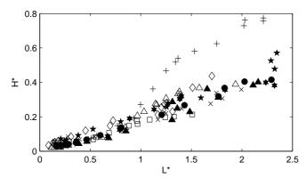
Fig. 7. Undimensional sheet cavity mean height  $H^* = H/H_{throat}$  according to the undimensional sheet cavity mean length  $L^* = L/H_{throat}$ :  $\times$ : plate 0,  $\bigstar$ : plate 1,  $\triangle$ : plate 2,  $\star$ : plate 3, +: plate 5, +: plate 6,  $\diamondsuit$ : plate 7,  $\square$ : plate 8.
