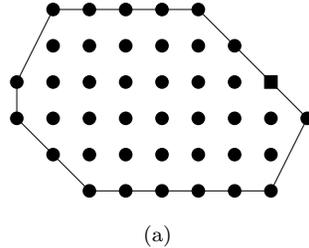
Figure 7: Convex hull of the discrete shape  $S$ : the point marked by a square is added during the application of Sklansky's algorithm. The discrete points belonging to the polygonal line are the vertices of  $Conv(S)$ .  $Conv(S)$  is defined as the discrete points inside  $Conv(S)$ .
