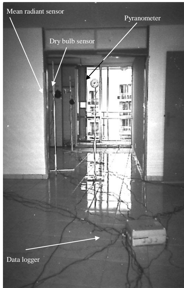
Fig. 10 : Monitoring of indoor short - wave radiation exchange
