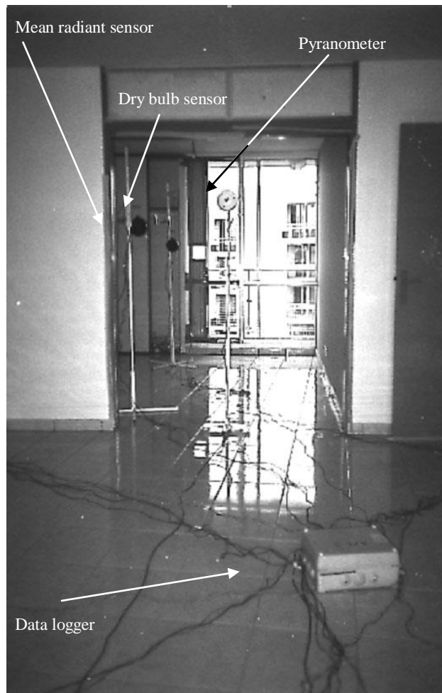
Fig. 10 : Monitoring of indoor short - wave radiation exchange
