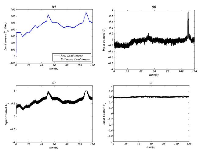
Fig. 9. (part 2). Tracking performances of the controller defined by (84a-d) in response to the varying wind speed of Fig. 7a.
