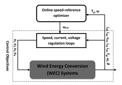
Fig. 5. Temporary state feedback controller for WEC system.
