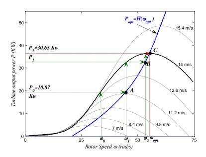
*Fig. 2*: Turbine Power Characteristics (Pitch angle beta = 0 deg).
