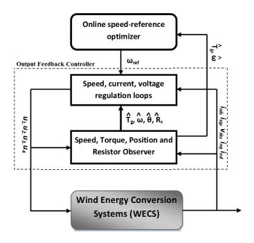
Fig. 3. Control system architecture for WEC systems
