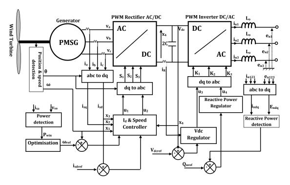
*Fig.* 6. Control system including AC/DC/AC converters and a synchronous aero-generator.
