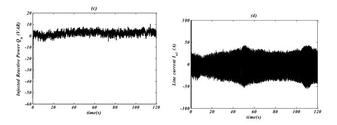
Fig. 8. (part 1). Tracking performances of the controller defined by (26), (32), (43) and (48) in response to the varying wind speed of Fig. 7a.
