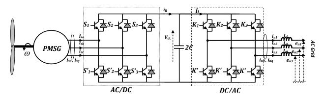
Fig.1. The AC/DC/AC Converter power circuit wind energy conversion system
