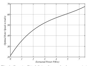
Fig. 4: Function F(.) defining the speed-reference optimizer
