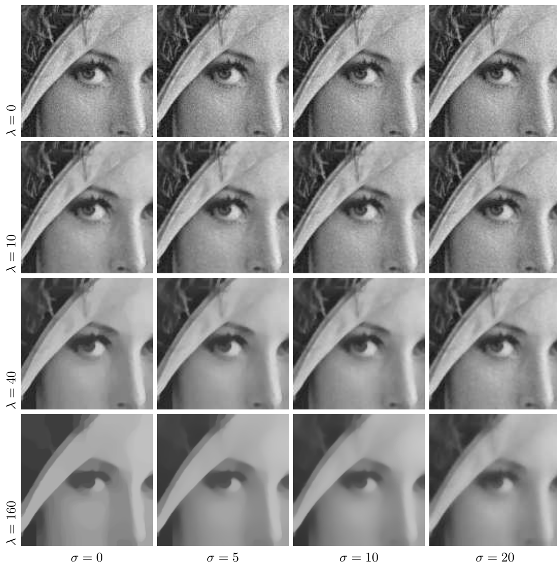
Figure 9: Effect of the two parameters \lambda and \sigma on TV-LSE. A noisy version of Lena image (Gaussian white noise with standard deviation equal to 10) is processed with TV-LSE for various values of \lambda and \sigma . First row: \lambda = 0 (the TV-LSE image is equal to the noisy image); second row: \lambda = 10 ; third row: \lambda = 40 ; last row: \lambda = 160 . First column: \sigma = 0 (the TV-LSE denoised image corresponds to ROF); second column: \sigma = 5 ; third column: \sigma = 10 ; last column: \sigma = 20 .
