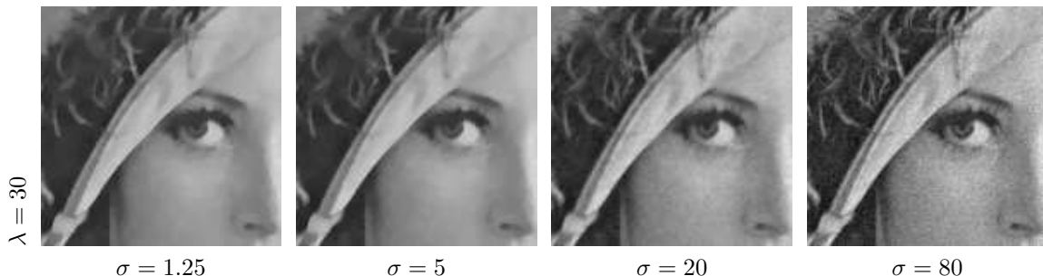
Figure 6: A noisy image is processed by TV-LSE with \lambda = 30 and increasing values of \sigma . When \sigma is small (left), the denoised image \hat{u}_{\text{LSE}} is very close to the MAP-denoised image \hat{u}_{\text{MAP}}(\lambda) , with some texture erased and some staircasing visible: the cheek and hat parts contain boundaries which do not exist in the original Lena image. As \sigma increases, \hat{u}_{\text{LSE}} looks more and more like the noisy image, which is consistent with the convergence \hat{u}_{\text{LSE}}(\sigma, \lambda) \rightarrow v when \sigma \rightarrow \infty .
