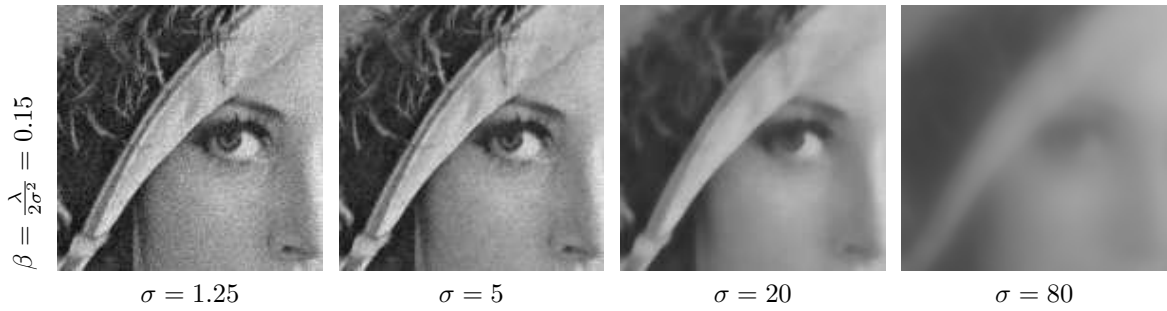
Figure 7: A noisy image is processed by TV-LSE with \beta = \frac{\lambda}{2\sigma^2} = 0.15 fixed and increasing values of \sigma . For small values of \sigma , the denoised image is close to the noisy image (left). As \sigma increases, the image is regularized, the edges are preserved but the texture is gradually erased. When \sigma further increases (right), the denoised image is completely blurred out.
