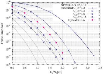
Fig. 10. The frame error rate of the proposed codes  $C_T$  for T=1,2,6 and hybrid nonbinary LDPC codes. It also shows the performance of rate half punctured mother code  $C_1$ . All these codes have 192 information bits. The curves labeled SP59 are the corresponding Shannon's 1959 sphere-packing bound [28]–[30] for rate 1/3, 1/6 and 1/18.
