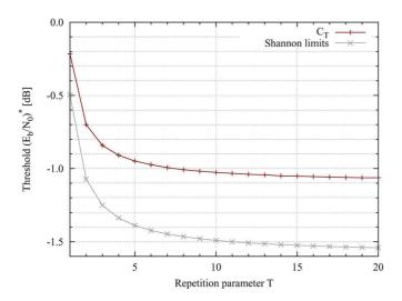
Fig. 8. The thresholds for the AWGN channels of the proposed codes  $C_T$  of rate 1/(3T) for  $T=1,\ldots,20$ . The codes are defined over  $\mathrm{GF}(2^8)$ .
