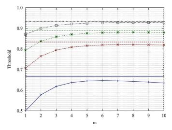
Fig. 5. Thresholds  $\epsilon^*$  of  $C_T$  over  $\mathrm{GF}(2^m)$  for the BEC and T=1,2,3 and 5 from below. The rate is 1/(3T). The straight lines show the Shannon limits 1-1/(3T).
