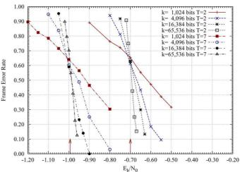
Fig. 9. Frame error rate versus parameter for the proposed codes  $C_2$  and  $C_7$  over GF( $2^8$ ) transmitting over the AWGN channel. The rates of  $C_2$  and  $C_7$  are 1/6 and 1/21, respectively. The information length are set to 1024, 4096, 16834, and 65536. The arrows indicate the corresponding threshold values. Observe how the curves move closer to these threshold values for increasing codeword lengths.
