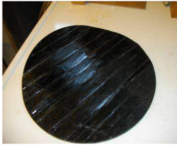
Fig. 2 Polymeric film side of B-GM
