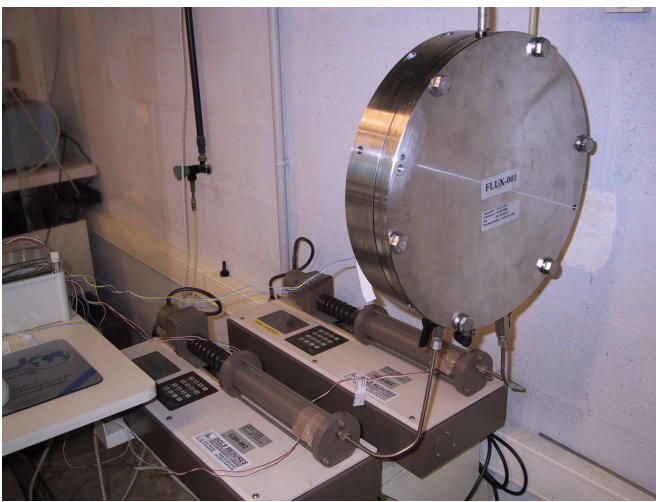
Figure 1 . View of the stainless steel cell and pressure volume controllers of type B device for flow rate measurement in geomembranes
