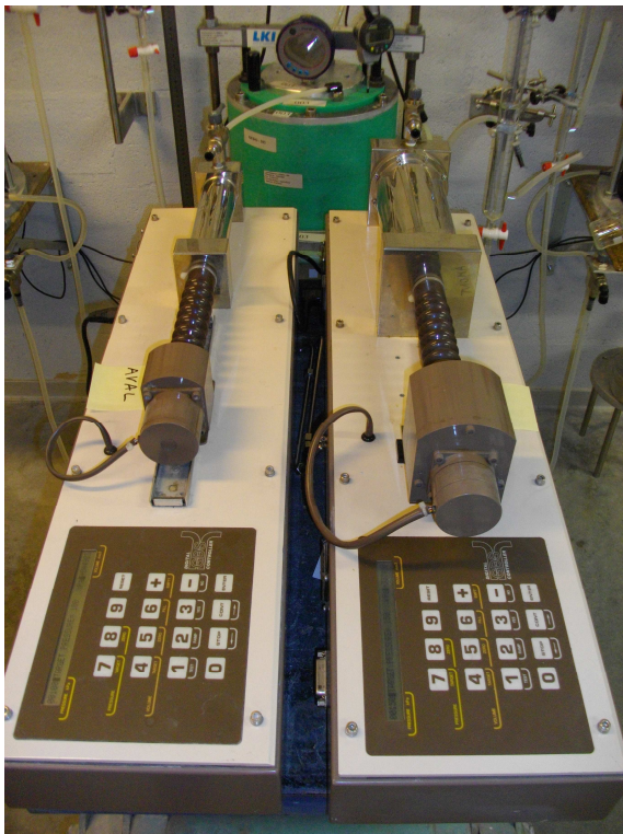
Figure 8. Experimental device for measurement of flow rates through multicomponent GCLs
