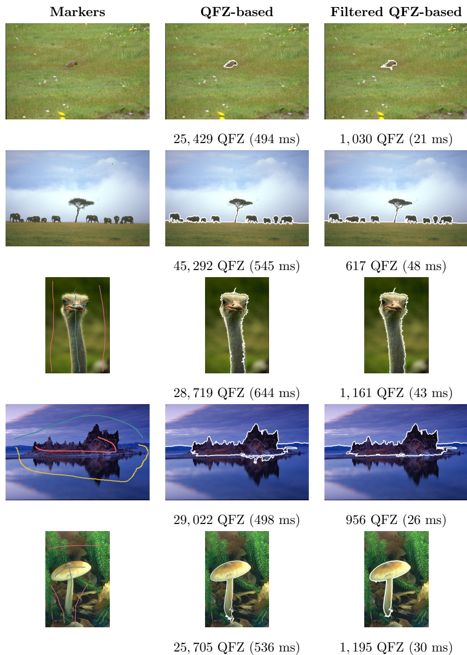
Figure 19: QFZ-based segmentation on sample images from Berkeley Dataset. Each segmentation is provided by the initial number of QFZ and the computation time required by the marker-based segmentation.
