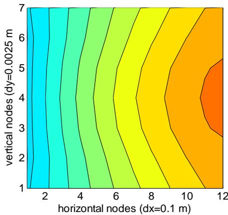
Figure 7: Melting degree of the PCM, point a
