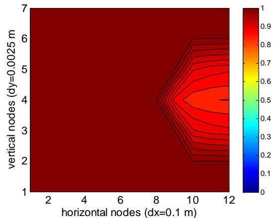
Figure 8: Melting degree of the PCM, point b
