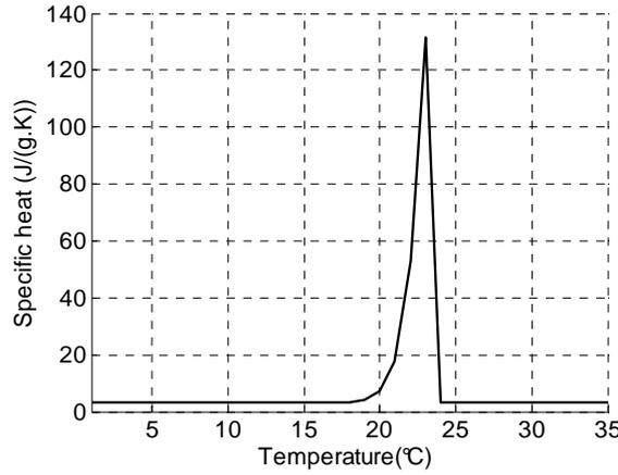
**Figure 3: Modeled specific heat of the selected PCM**
