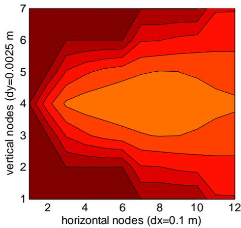
Figure 9: Melting degree of the PCM, point c
