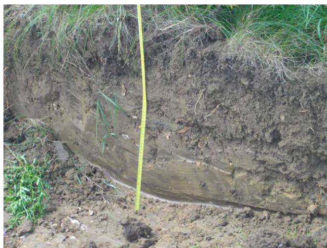
Figure 1. Landfill cover layer.
