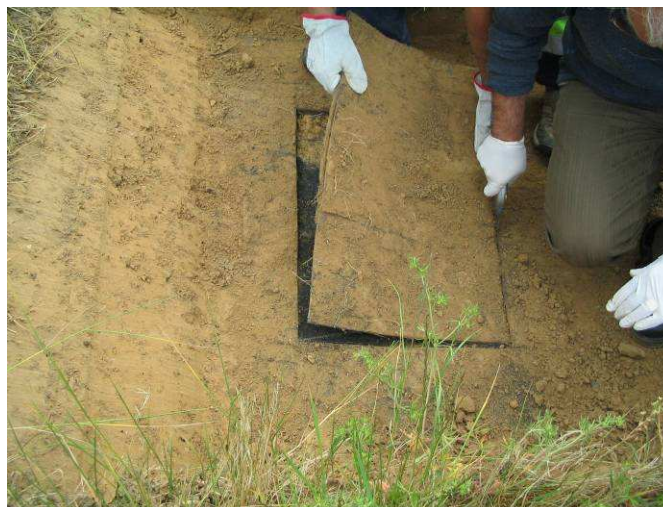
Figure 3. Exhumation of GCL samples.
