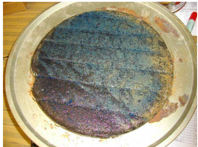
Figure 4. GCL specimen after test with the blue dye.
