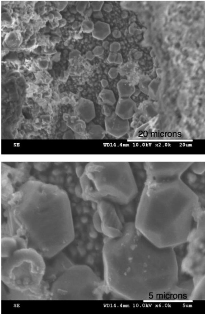
Fig. 16. SEM observations of newly formed CaCO<sub>3</sub> crystals (SE detector for the image, BSE detector+EDS analysis for mineralogical composition of crystals) inside a capillary pore of Haubourdin chalk heat-treated up to 500 °C. It clearly corresponds to the inside of a hollow micro-fossil, with incipient cementation, either due to heat-treatment or to diagenesis. No such crystals have been observed on 60 °C oven-dried chalk.
