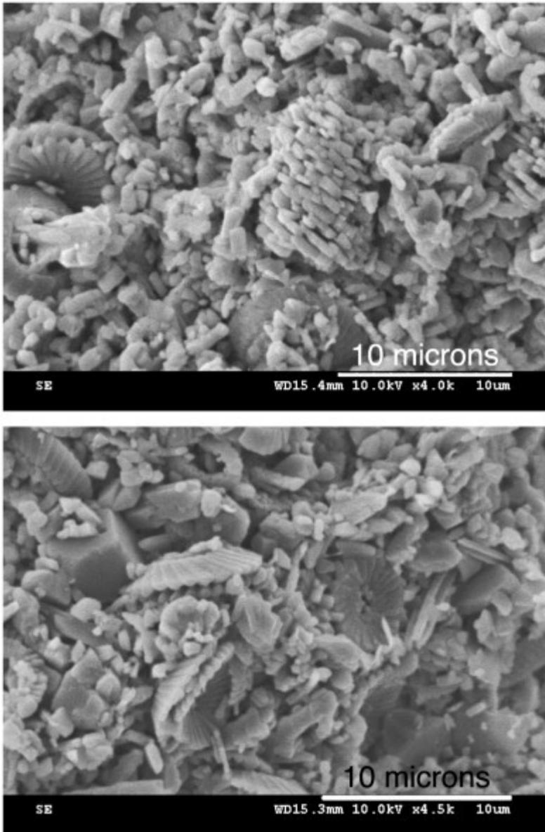
Fig. 2. Observations of 60 °C oven-dried chalk without epoxy resin impregnation, using the SEM/SE detector. These show entire coccolith disks, and (center of top image) the imbrication between calcite grains (which constitute the coccoliths), or (top left of bottom image) several angular calcite crystals, for which chemical composition is proven by EDS analysis.
