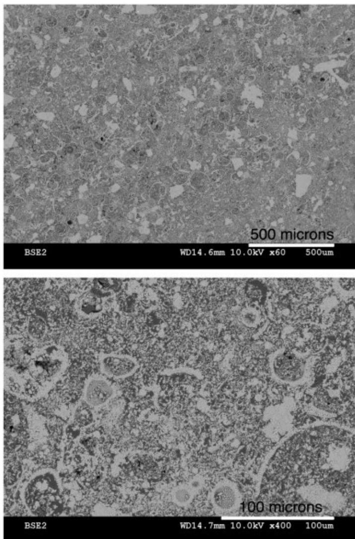
Fig. 5. SEM observations of Haubourdin chalk after epoxy resin impregnation and polishing, using the BSE detector after 500 °C heat-treatment for 48 h.
