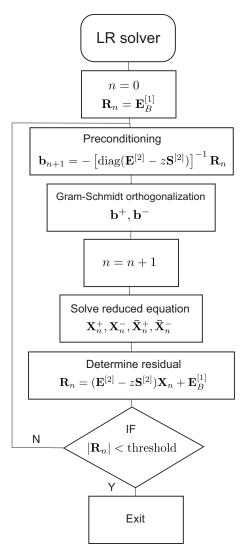
FIG. 1. Flowchart of the linear response equation solver.
